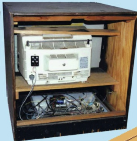
» Usually a stripped down television, single game board, and a power supply were all that resided inside machines.
